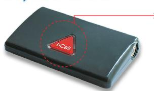
Press the bCall button once to check on device battery status
